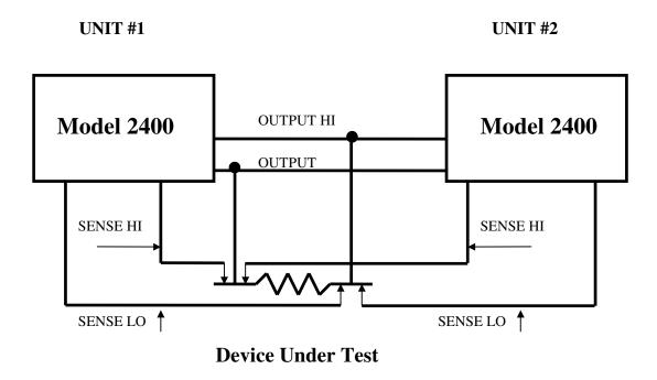
Figure 1. Connecting two Model 2400s in parallel
